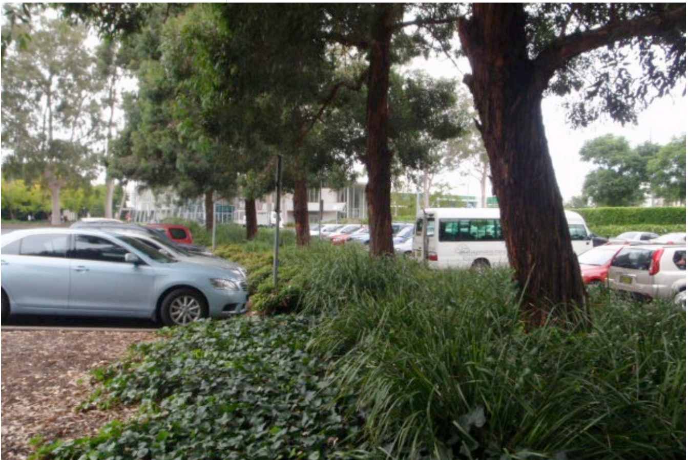
Median planting and shade trees in between rows of car parking provides shade, reduces hard paved areas, heat absorption and radiation and reduces stormwater run off (Photograph: Penrith City Council)
